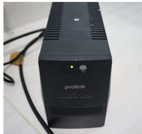
Uninterruptable Power Supply (UPS)
